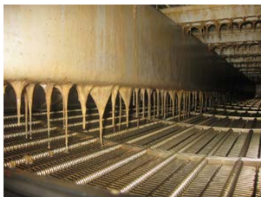
Pasteurizer after one week without chemical treatment
